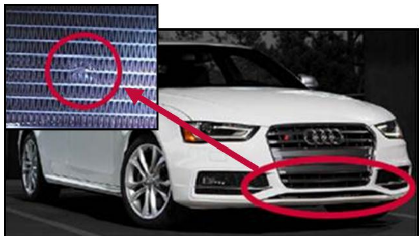
Figure 1. Damage from front-end stone impact.
