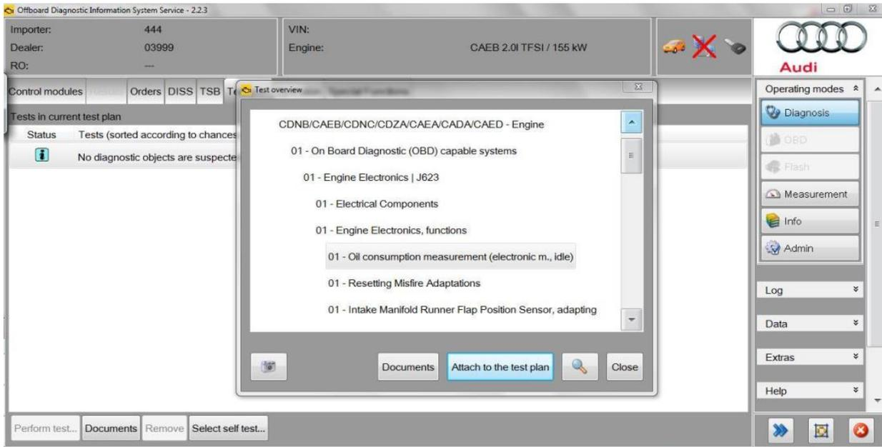
**Figure 1.** 01 – Oil consumption measurement (electronic measurement).
