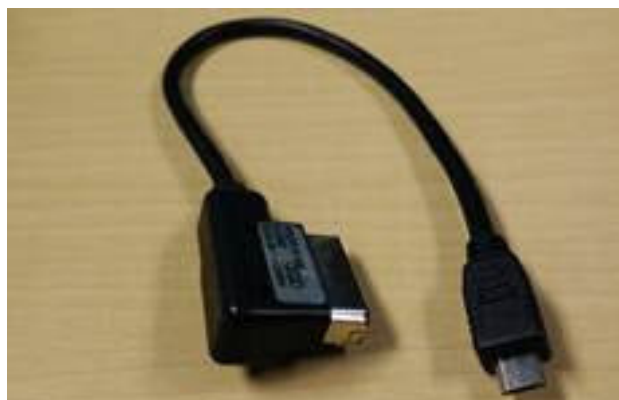
Figure 6. Male Micro USB AMI cable that can be plugged directly into the phone.
