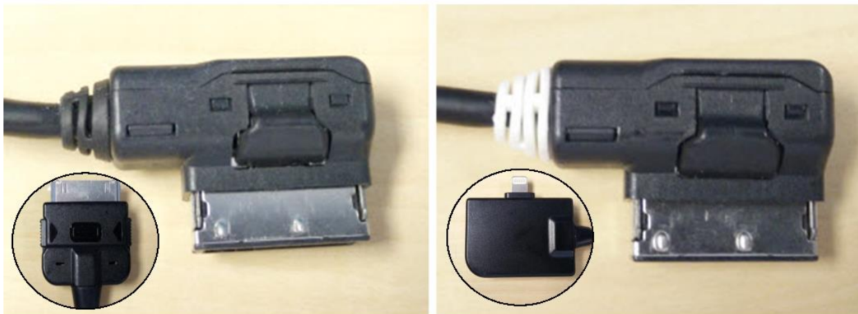
Figure 1. From left to right: Black grommet cable with Apple 30-pin dock connector and white grommet 8-pin AMI Lightning™ adapter cable.
