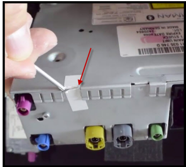
Figure 6. Break white warranty seal.
