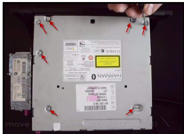
Figure 5. MMI main unit with screw locations for top cover indicated by the red arrows.
