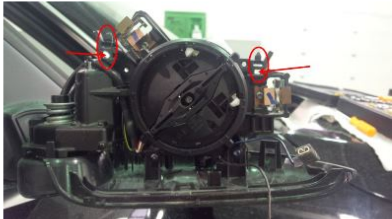
Figure 2. Exterior rear view mirror glass and housing removed. Retaining clip engagement locations are shown.
