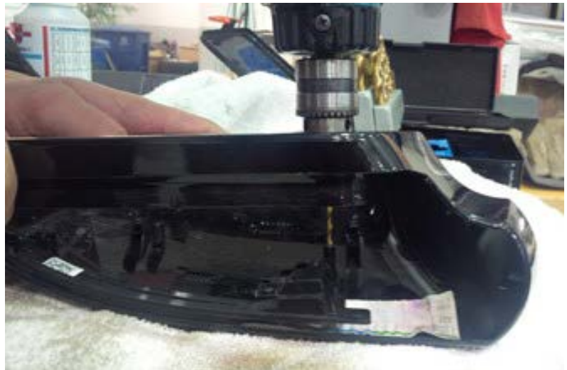
Figure 5. Drilling out the boss opening to 3mm.
