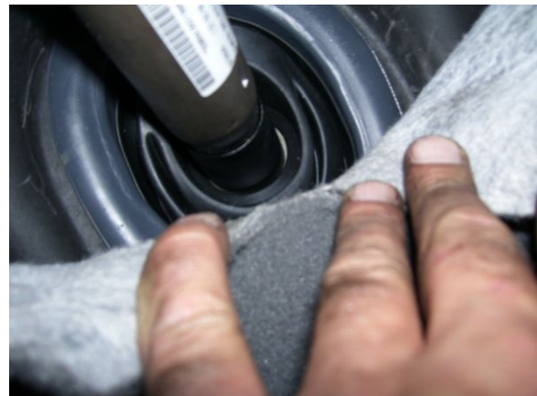
Figure 1. Sealing sleeve on the bulkhead.
