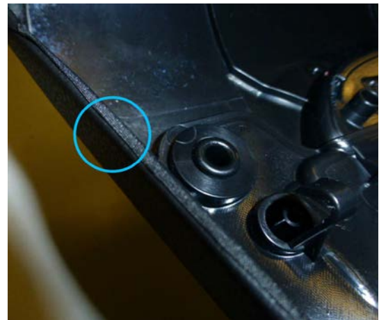
Figure 2. Correct application of textile adhesive tape.
