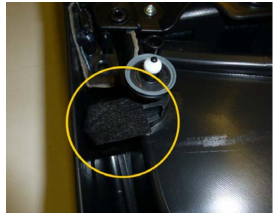
Figure 3. Correct application of felt strip.
