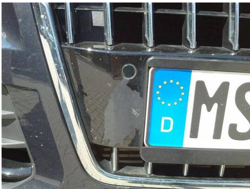
Figure 1. Example of flaked-off paint.
