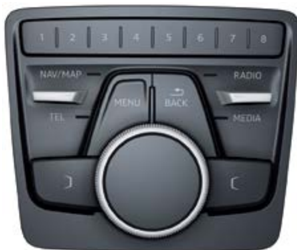
"Mid" control panel with automatic transmission
