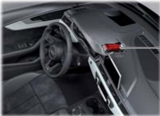
Electronic Steering Column Lock Control Module J764
