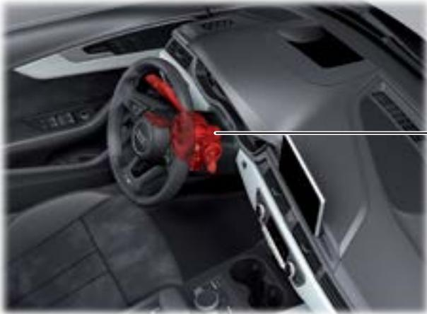
Steering Column Electronics Control Module J527
