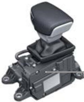
Selector Lever Sensor System Control Module J587
