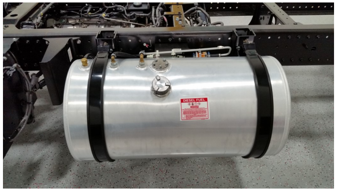
Auxiliary Fuel Tank
