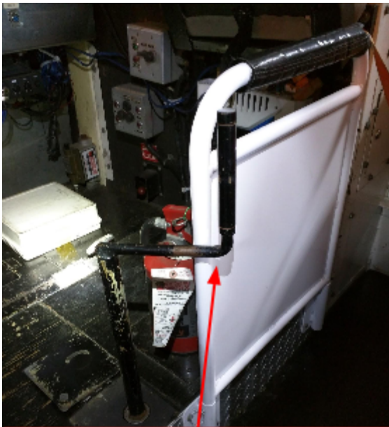
PHOTO #1 EMERGENCY STEERING ARM CONTACT WITH PASSENGER WALL
