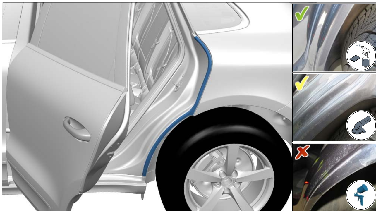
Checking and evaluating paint surface
