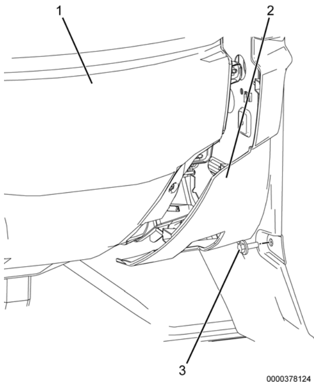
Figure 1. Floor Duct Trim Panel.
