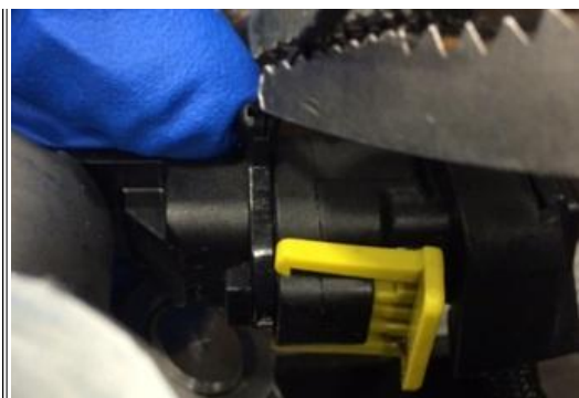
Figure 12: Wire Tie the Connector Clip
