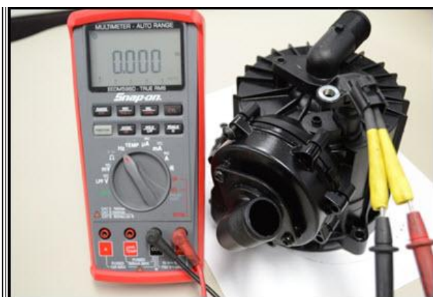
Figure 4: Digital Multimeter Hookup
