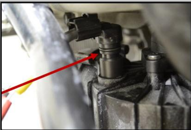
Figure 3: CMP Sensor with electrical tape installed
