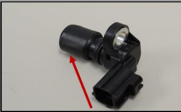
Figure 2: CMP Sensor with electrical tape installed
