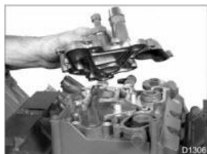
Figure 338. Removing oil filter base assembly
