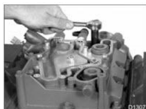
Figure 339. Mounting bolts for oil cooler cover assembly
