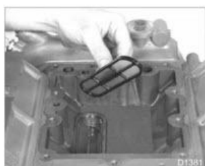
Figure 341. Pump inlet strainer
