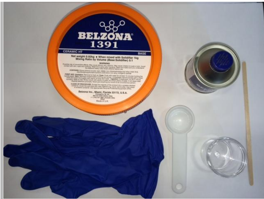
Figure 21: Belzona 1391 Epoxy Mixing Supplies
