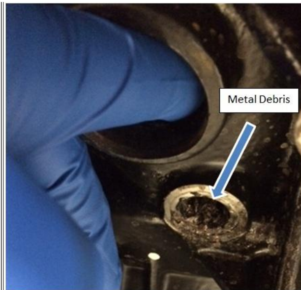
Figure 14: Metal Debris Removal
