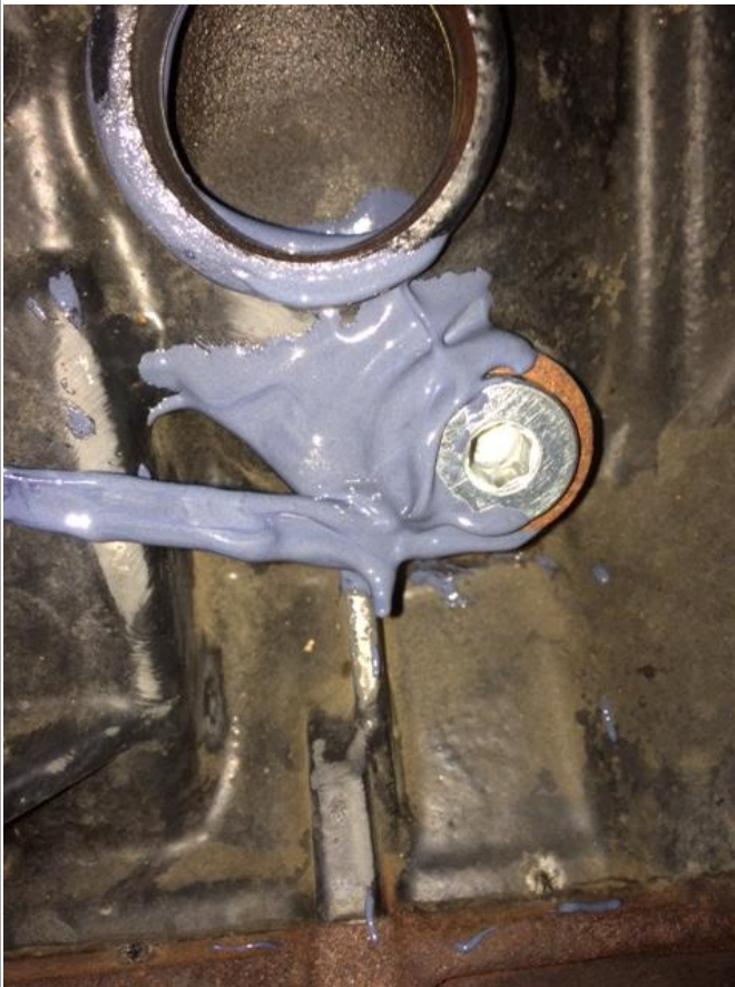
External Figure 3: Paste epoxy on the outside of the engine block
