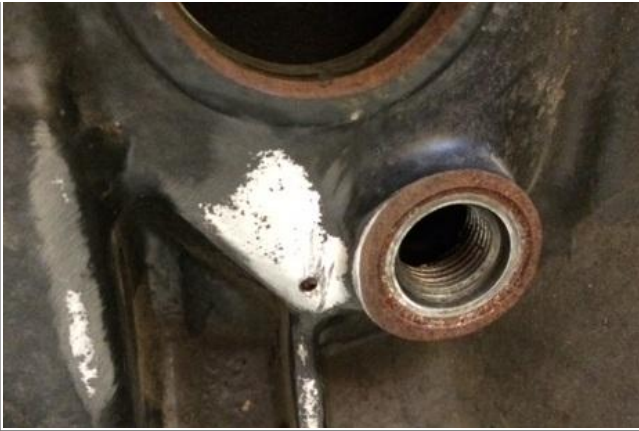
External Figure 1: External Leak Paint Removed
