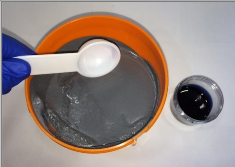
Figure 23: Clean Tablespoon to Measure Epoxy Base (3 Tablespoons)
