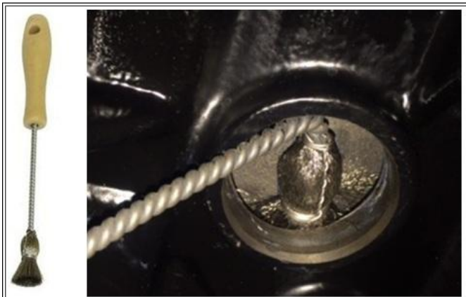
Figure 16: Using ZTSE4391 to scrub the cavity
