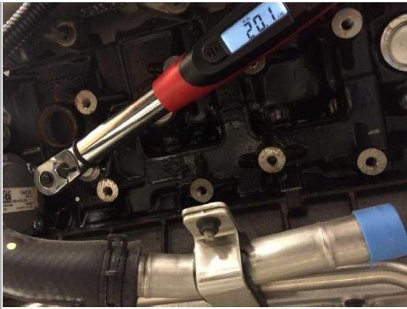
Figure 20: Install and Torque New Hex Plug
