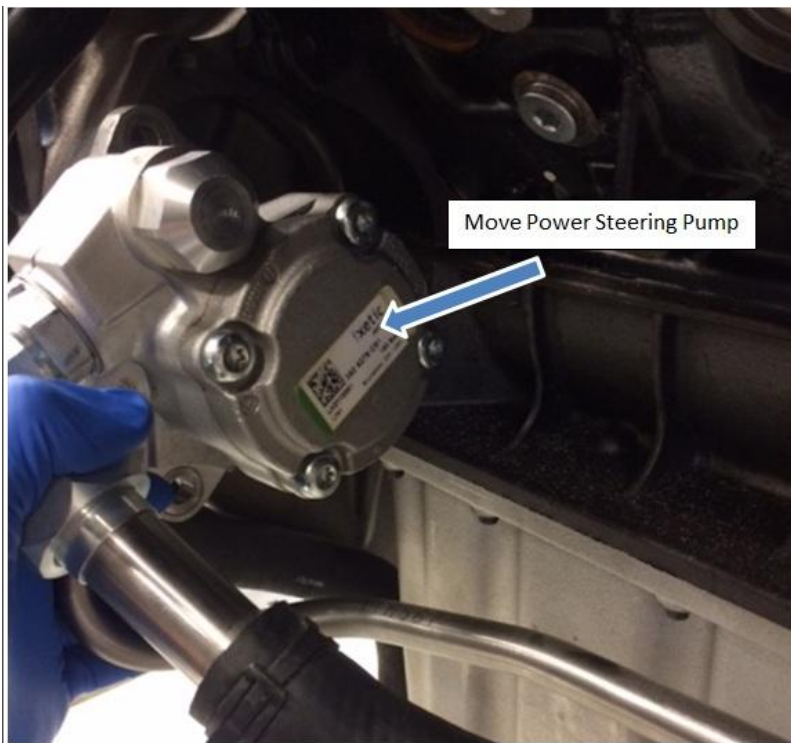
Figure 8: Move Power Steering Pump Away from Working Area
