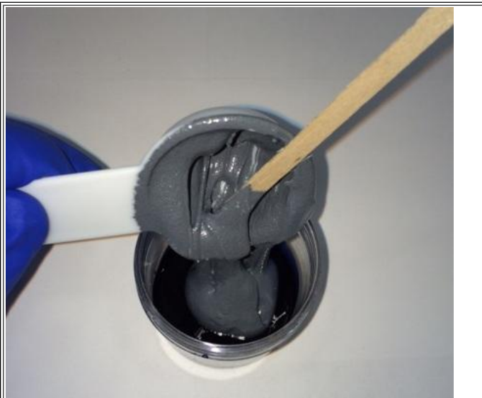
Figure 24: Scrape Epoxy Base into Mixing Cup
