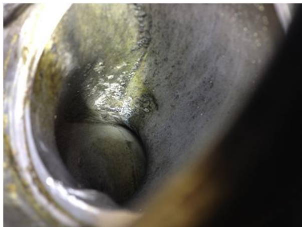
Figure 1: Porous HP turbocharger air inlet duct leaking coolant into the intake.
