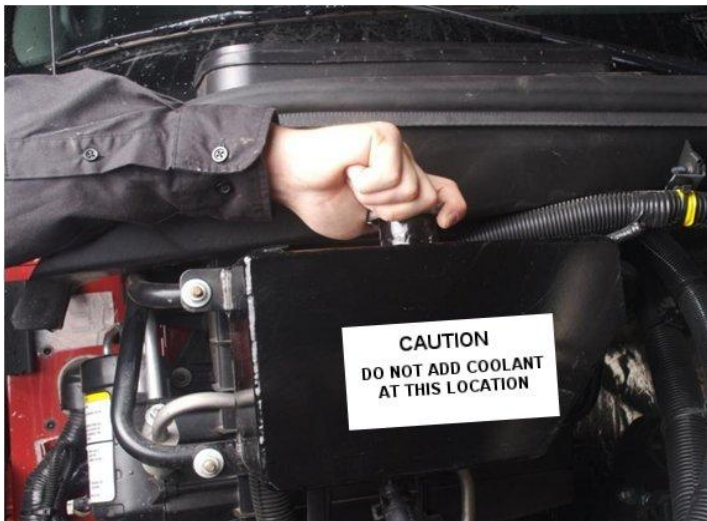
Figure 1 - Pressure Cap Installed on Expansion Tank
