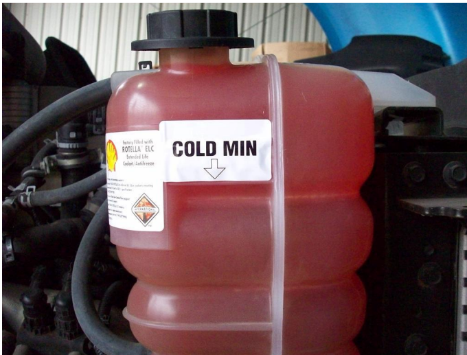
Figure 8 - Adjust coolant level and install NON VENTED Cap
