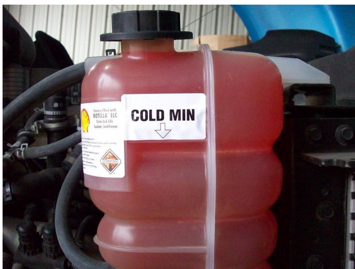
Figure 8 - Adjust coolant level and install NON VENTED Cap
