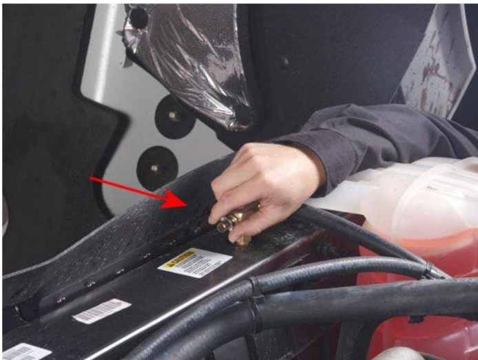
Figure 5 - Close air bleed on the top tank of the HTR
