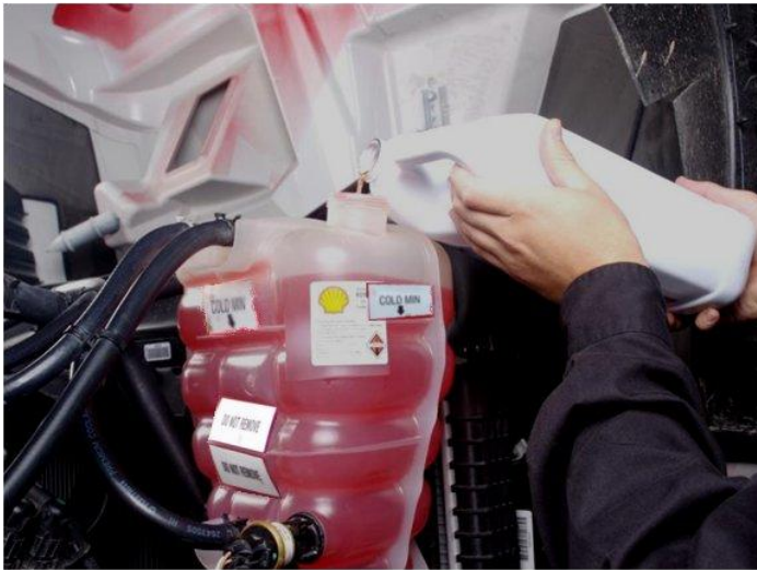
Figure 6 - Fill cooling system at deaeration tank (Fill to top of tank)
