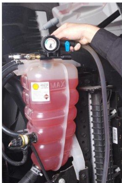
Figure 7 - Install Vacuum Fill Tool
