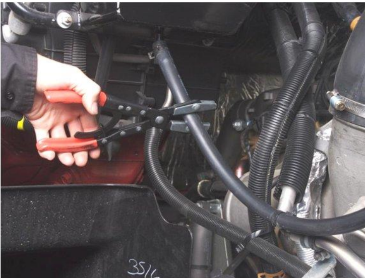
Figure 2 - Clamp expansion tank hose with hose clamp off tool.
