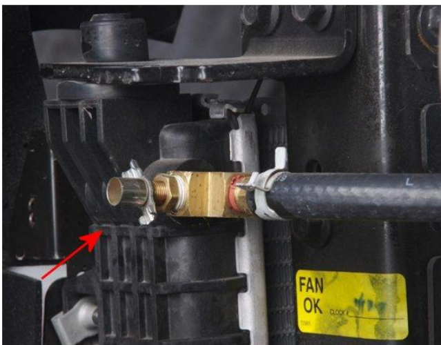
Figure 6 - Close the air bleed on the LTR ( Low Temperature Radiator)
