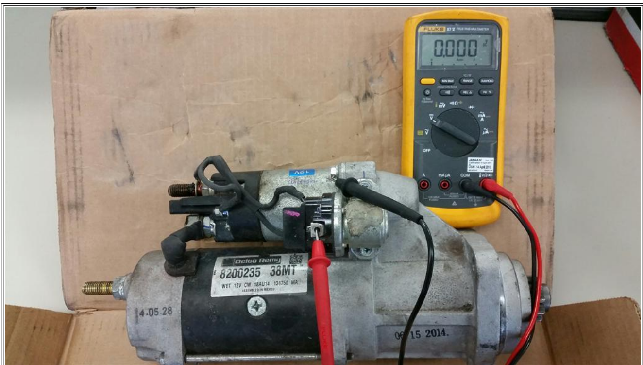
Figure 1: Starter IMS S terminal DVOM Hookup Location
