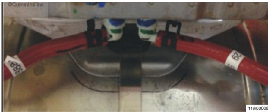
Figure 5: Correct DPF differential pressure sensor orientation with marking from previous incorrect orientation
