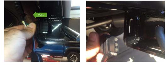
3) Using slack in harness, pull the connector from under the bumper cover and connect to the trailer's harness.
