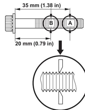
14. Apply new oil to the connecting rod bolt threads and flanges. Torque the bolts to **20 N·m (14 lb-ft)**, then tighten the connecting rod bolts an additional **90 degrees**.
