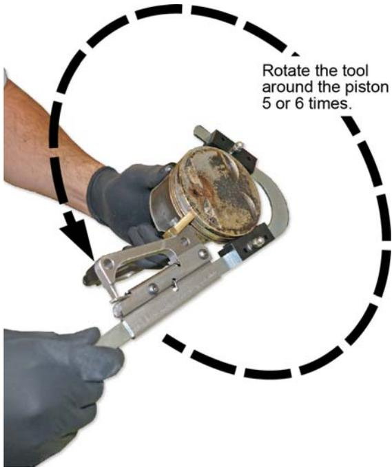
7. Remove the piston groove cleaning tool and clean off the carbon from the tool bit.
