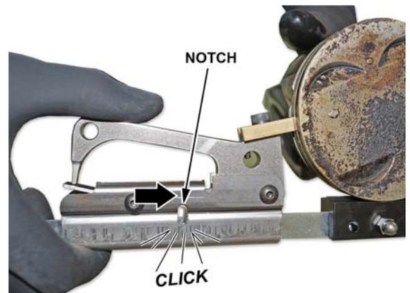
6. Hold the piston steady and rotate the tool counter-clockwise five to six times to remove any carbon deposits in the piston ring grooves. **Do not** rotate the tool clockwise.
