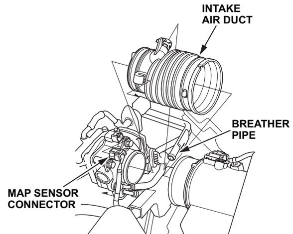
19. Disconnect the throttle body connector, the EVAP canister purge valve connector, the EVAP hose, the brake booster vacuum hose, and the vacuum hose.
