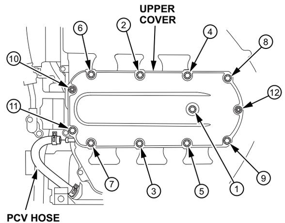
30. Remove the intake manifold bolts and nuts in three steps, then remove the intake manifold.
