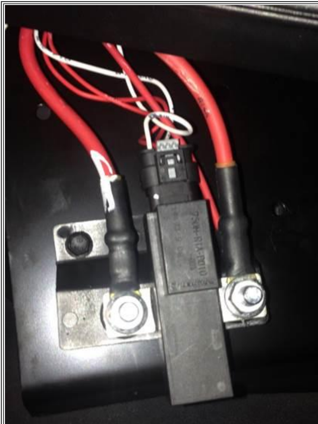
Figure 1: Load Shed Relay - Correct Wiring Configuration.
