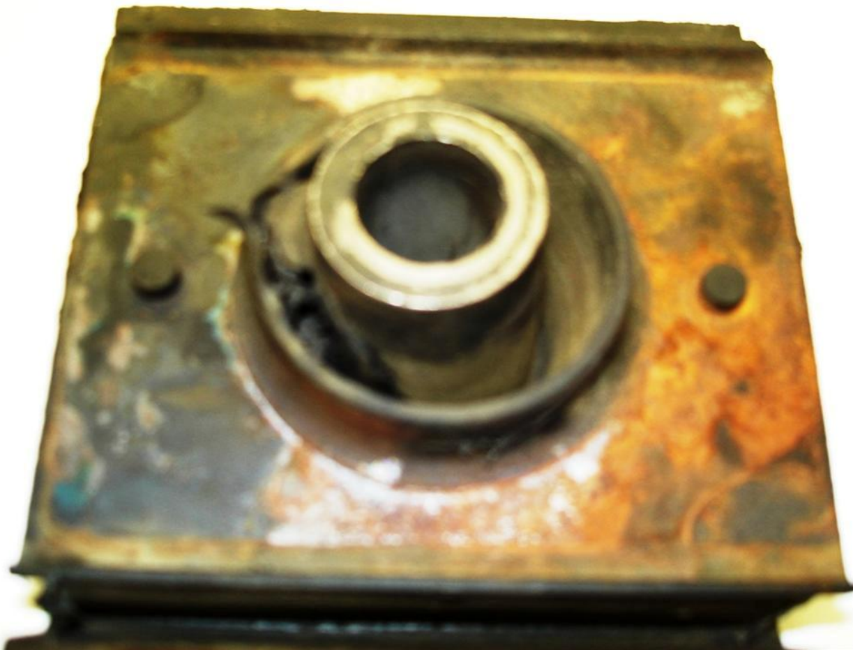
Figure 2: FRONT INSULATOR DAMAGE
