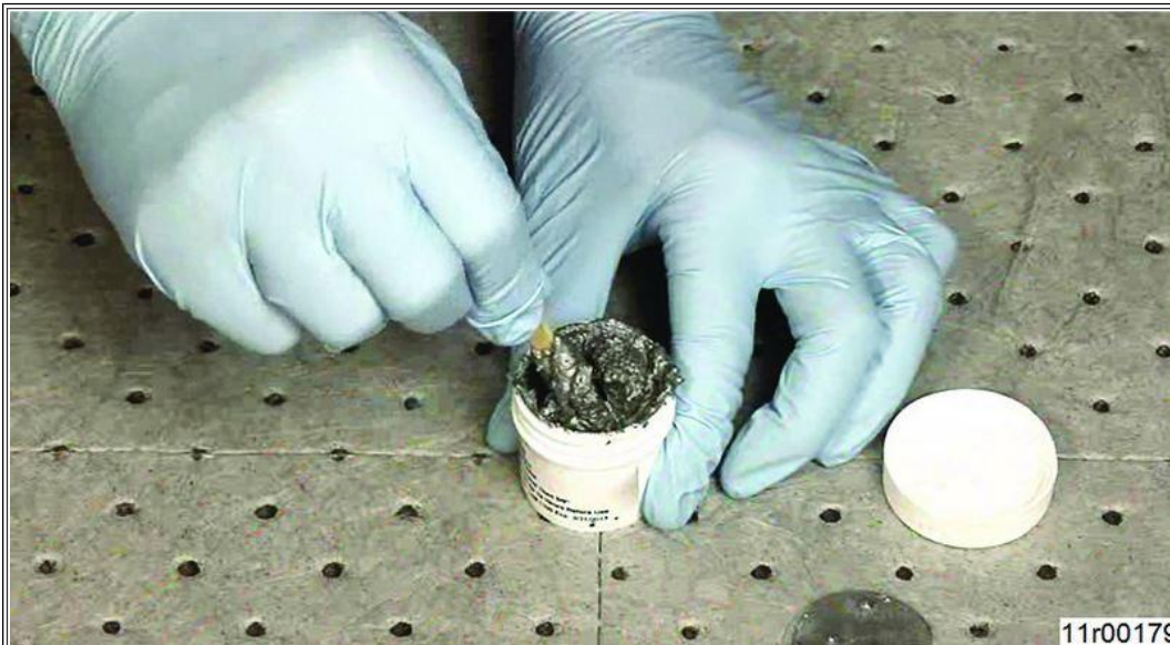
Figure 10: Mix High Temp Sealant
