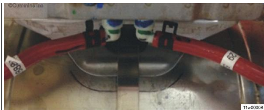
Figure 5: Correct DPF differential pressure sensor orientation with marking from previous incorrect orientation
