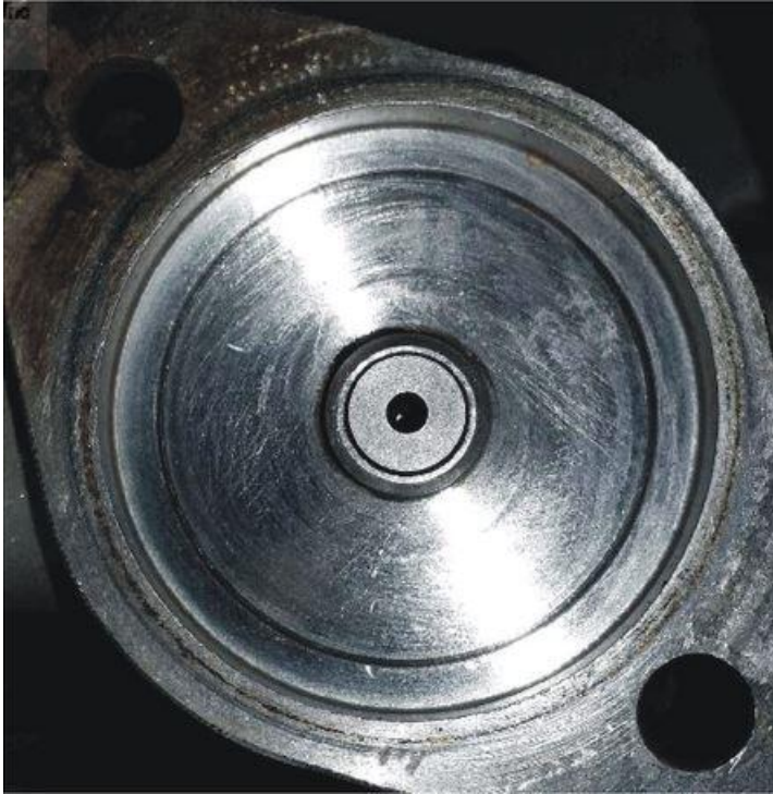
Figure 1: Missing Poppet - EcoFit™ Aftertreatment Fuel Injector
