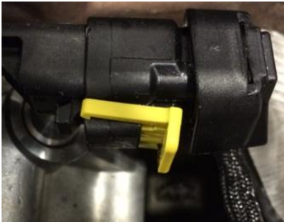
Figure 5: Fully Seated PCV Connector with CPA Disengaged
