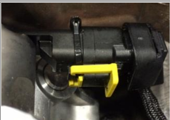
Figure 7: Reengaged CPA (Completed)
