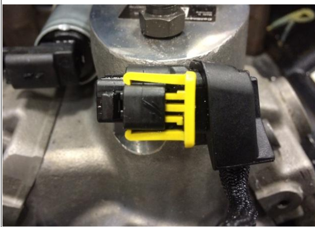
Figure 3: Fully Disengaged CPA
