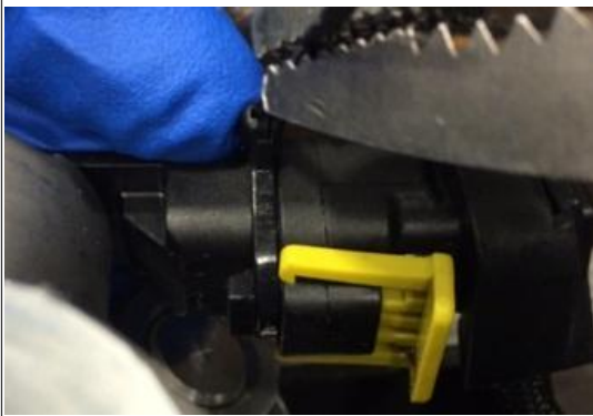
Figure 6: Wire Tie the Connector Clip
