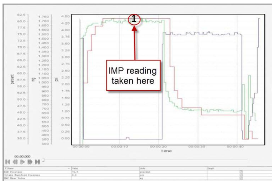
1. Intake Manifold Pressure (IMP)
