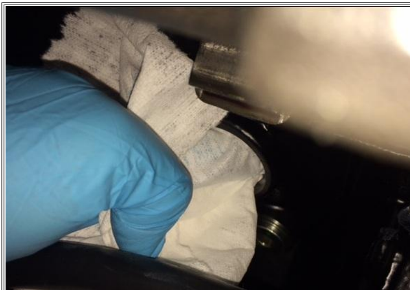
Figure 17: Wiping the cavity clean
