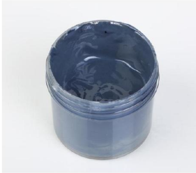
Figure 25: Fully Mixed Belzona 1391 Ceramic Epoxy
