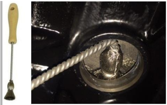
Figure 16: Using ZTSE4391 to scrub the cavity
