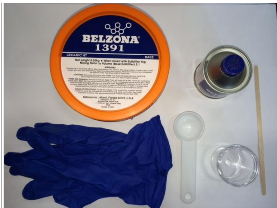
Figure 21: Belzona 1391 Epoxy Mixing Supplies
