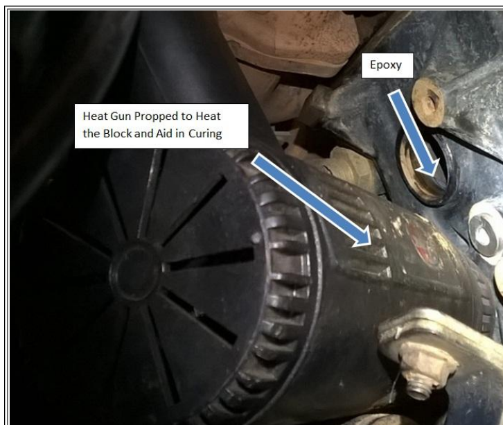
Figure 28: Use a Heat gun to Cure the Epoxy
