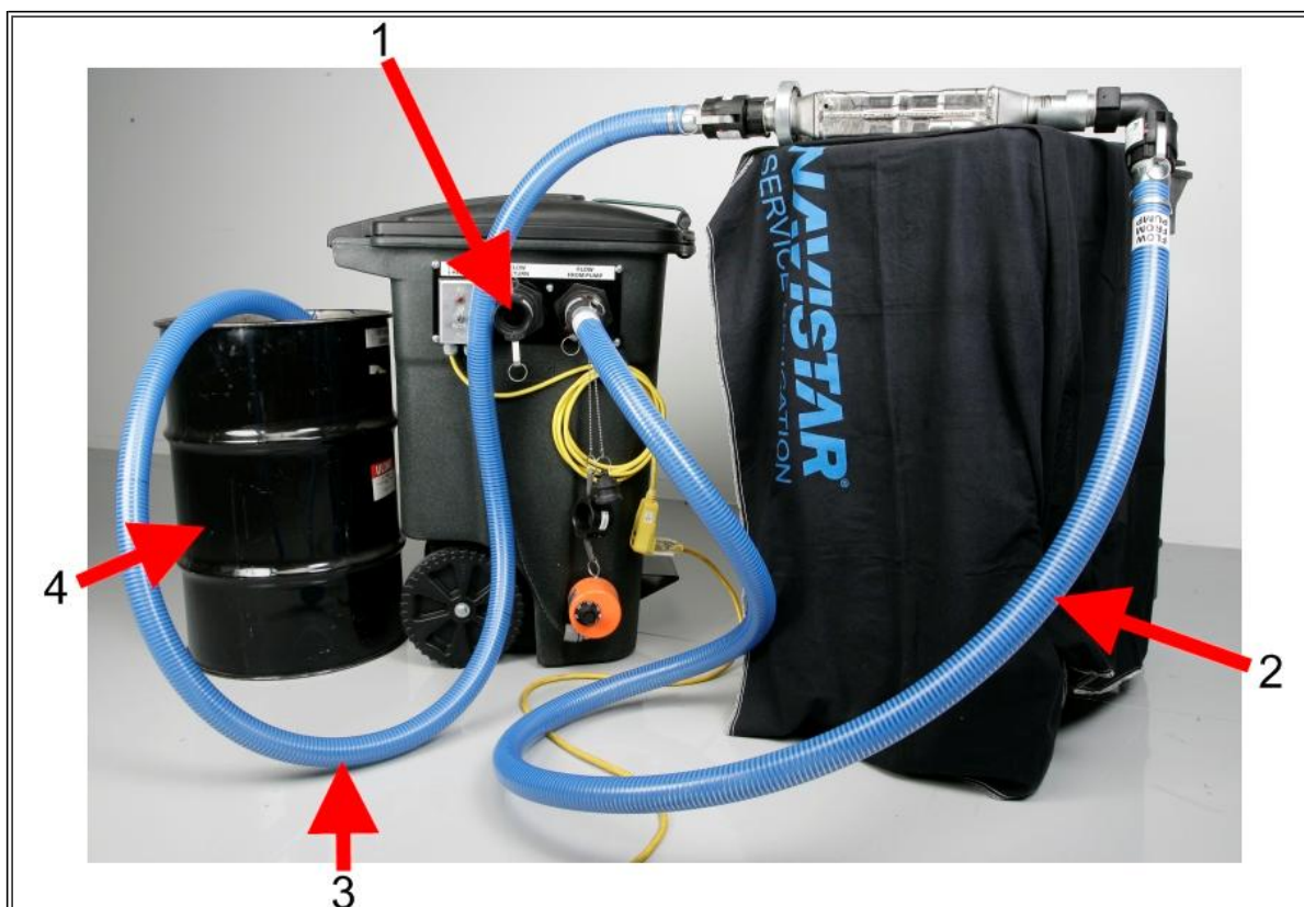
Figure 17. Draining Cleaning Management System (12-353-01A)
