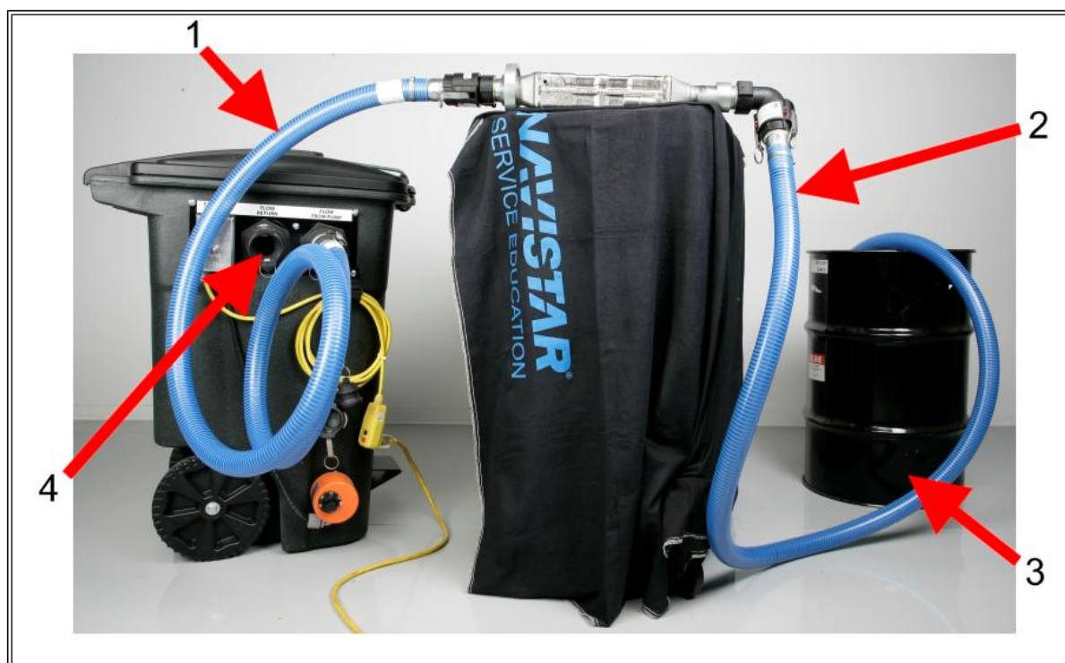
Figure 19. Draining Cleaning Management System (12-353-01A)
