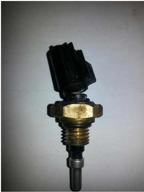
Figure 1: Damaged CACOT Sensor
