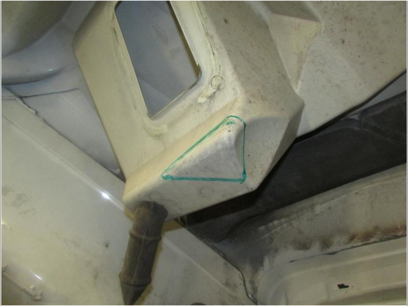
Figure 6: Template traced on air inlet duct.
