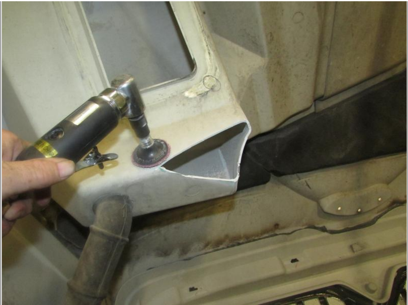
Figure 8: Sanding/roughing of the patch area.
