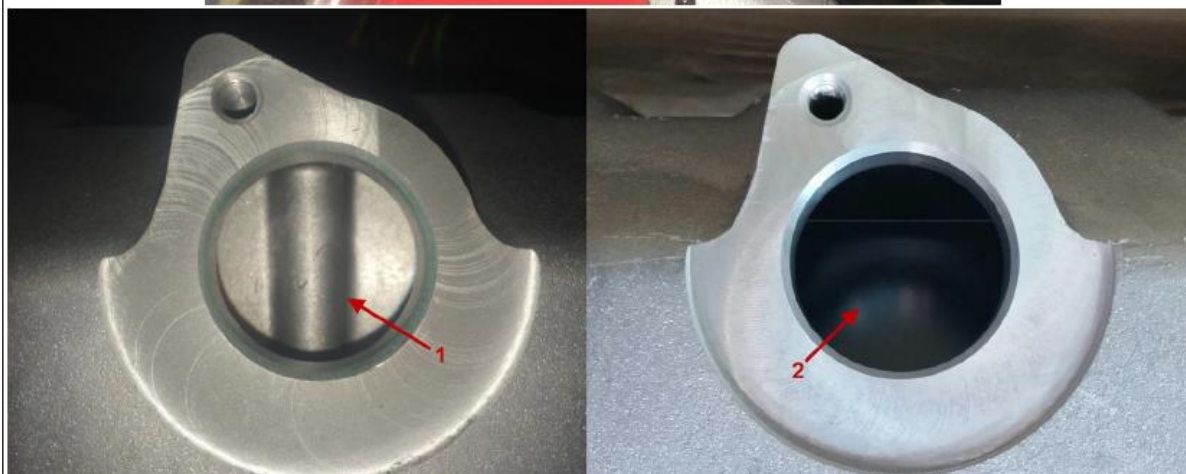
Figure 1: Valve cover baffling vs non-baffled
