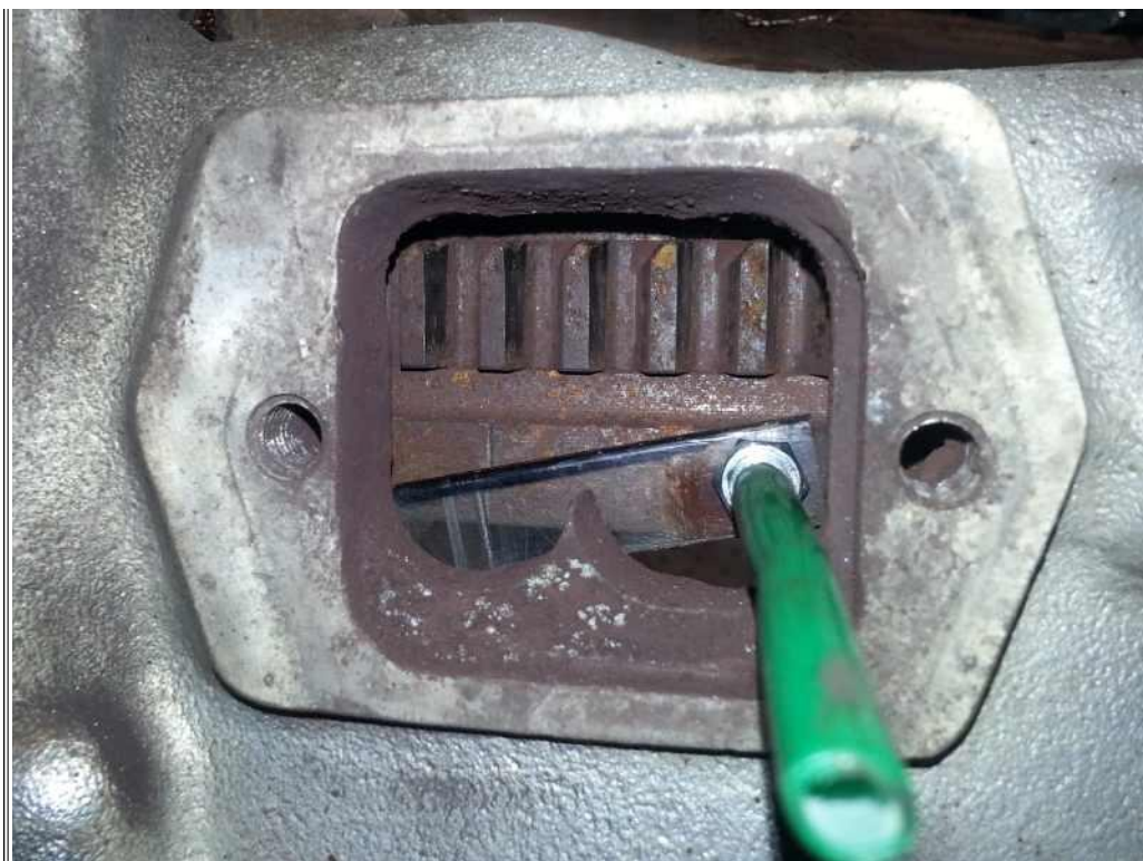
Figure 2: Flywheel Timing Tool Installed
