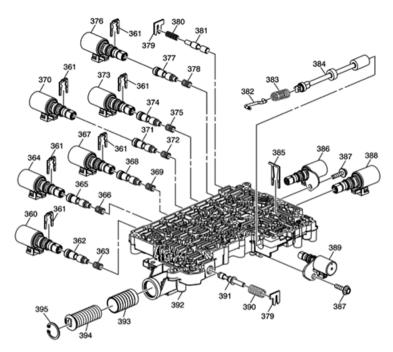
(361) Control Solenoid Valve Retainer
