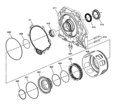
(414) Propeller Shaft Transmission Flange Fluid Seal (Outer)
