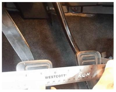
Measure from the top of the brake pedal pad to the straight edge on the Left side of the brake pedal as per A above, Then measure the Right side of the brake pedal to straight edge as per B above. You should have no more than +/- 2mm from side to side measurements. Any more than that will require replacement of the pedal assembly.
