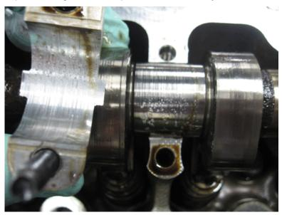
3. Inspect the timing chain idler sprockets for stiffness when turning. ( Should turn smooth and free)
