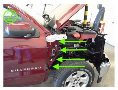
To repair, apply clear flowable seam sealer to the cowl seam (3) and into the pocket (4 & 5) as shown below.
