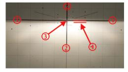
Note: GMC Sierra Low beam pattern (1 Lamp) on wall/aiming screen at 25 ft (7.62 m)
