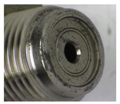
If additional magnetic debris is found on the Fuel Rail Pressure Sensor and/or Fuel Pressure Regulator 2 (Pressure Relief Valve) the Fuel Injection Pump is experiencing the condition described.
