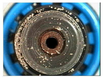
The pictures above are examples of Pressure Regulator 1 with the magnetic debris described
