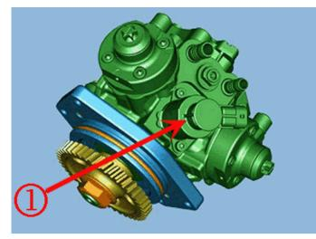
Remove the Fuel Injection Pump / Pressure Regulator 1 for inspection.
