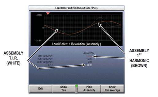
The GSP9700 is set to display T1 RFV. Higher order RFV, T2 & T3 can be displayed in the Assembly Data Plots Screen, as shown above. Depending on the level of GSP9700, the screen may be under 'Data' or 'Runout Plots,' then "Rim and Load Roller Runout Plots."
