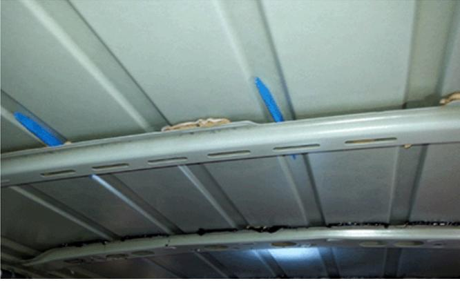
5. Apply the panel vibration control material (as listed below), in an in-out / zig-zag pattern while working along, to fill the voids between the roof bow and sheet metal, on both the front and rear sides of the bow. In some cases, it may take a couple layers of material to fill the void.
