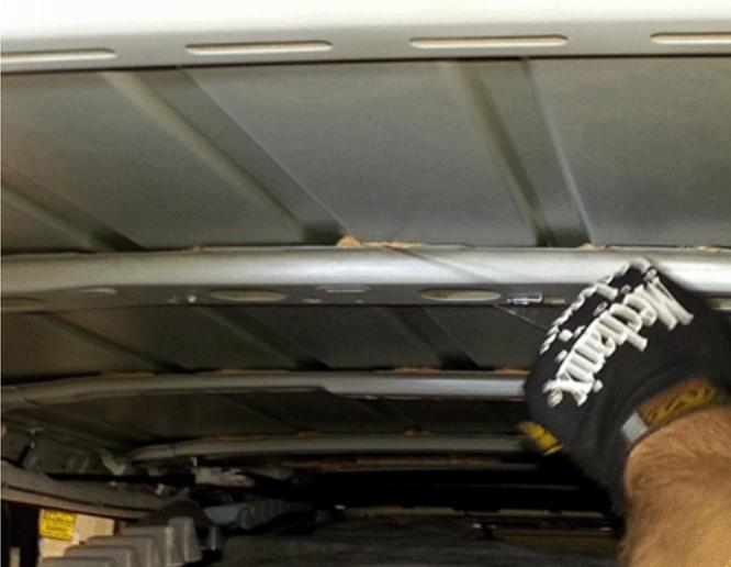
3. Position a trim stick, thin side up-down in the reinforcement rib on either side of the middle roof sheet metal rib.
