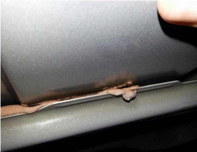
To correct this concern, remove the old bonding material, and apply panel vibration control material between the roof bows and roof sheet metal.
