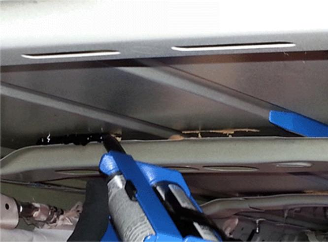
6. Rotate the trim sticks, from tall to thin side up-down and remove the trim sticks.
