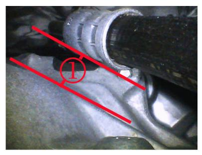
When bending the line, care should be taken to not kink the line or unseat the pass-through grommet (Indicated by the arrows in the image below); a small screwdriver handle or similar instrument wedged between the line and vehicle under body tunnel structure may be useful in creating leverage to bend the line without unseating the grommet.
