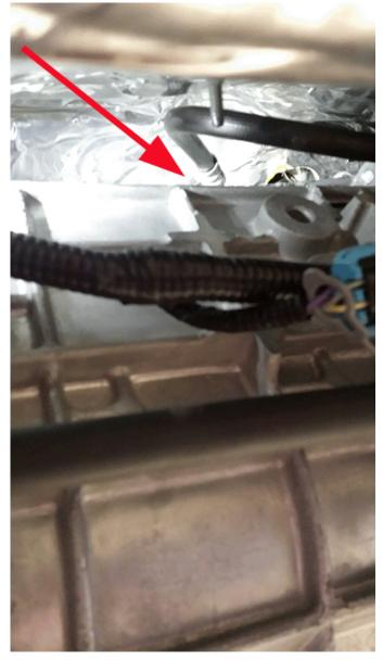
h. Reposition the clutch release line by bending it toward the passenger side of the vehicle to create a 1/2" (13mm) gap between the line and transmission as per the number 1 indicated in the picture below.
