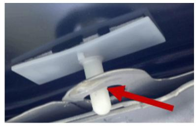
The windshield alignment pins are in the upper corners of the glass.
