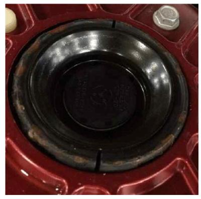
This concern is not actually rust, rather, is caused by an applied layer of rubber to the top of the strut that does not completely cover the nylon underneath. This appearance will not affect performance or durability of the vehicle. It is strictly a cosmetic concern..
