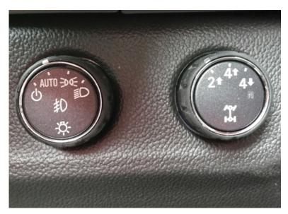
For Canyon (NQ6): Before performing Service Information diagnostics verify that the vehicle has the correct 4WD switch installed in the dash panel.
