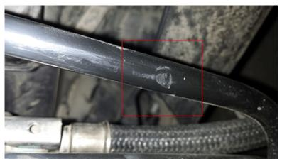
Replace PCV dirty air tube and cover it with conduit to protect from repeat damage. Reset idle and fuel trim retest for the concern.
