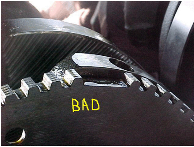
Crankshaft with bad reluctor wheel
